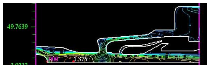
Simulation of air flow field: distribution of Mach number at a certain time of interrupters breaking
